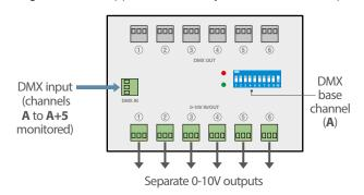
The diagram below shows the inside story of the DMX to 0-10V conversion. Six channels, in this case 4 thru 9, of the DMX input are converted into equivalent analog values.
