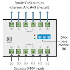
The diagram below shows the inside story of the 0-10V to DMX conversion. The six separate 0-10V inputs are converted into equivalent digital values (each between 0 and 255). These are then applied to the six DMX channels that are selected by the switch block -
