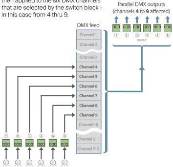
The complete DMX universe (including the six affected channels) is duplicated across all six of the DMX Out ports. Each port can drive up to 32 DMX devices. Note: The output values for all other DMX channels (apart from 4 thru 9) will remain at zero.
