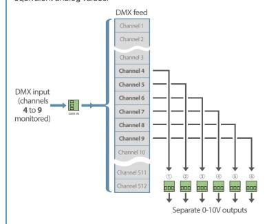
The analog values are then applied individually to the six 0-10V output ports. Each port can drive one 0-10V current sink device.
