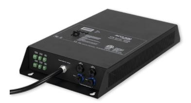
XTR Driver 4000™ is a specialized module that powers continuous runs (up to 700′/213m) of high intensity linear LED fixtures. XTR Driver 4000 features a 220V-277VAC power input, a clear display for control input selection and up to 4000W of high voltage DC output power. The following control formats are all supported: DMX-512A, DALI or 0-10V/1-10V. All connected linear LED fixtures must conform to the Acclaim Lighting XTR Link standard.
