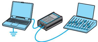
If the XMT-350 is connected to a PC, the DMX input port might be a **ground referenced receiver** when the USB is grounded.
