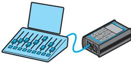
If the XMT-350 is battery operated, the DMX input port is an **isolated receiver**.
