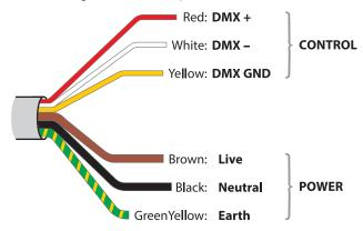
Control cores: 24 AWG / 0.25mm<sup>2</sup> **IMPORTANT: Ensure that power earth**Power cores: 14 AWG / 2.5mm<sup>2</sup> **IMPORTANT: Ensure that power earth**and **DMX GND are both tied to true earth.**
