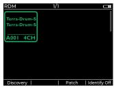
3 Highlight the Terra Drum fixture and press ✓ to view the fixture details:
