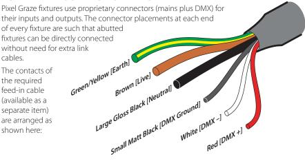
Note: Ensure that the mains power is supplied from a suitably protected source and initial connections are made within IP rated enclosures.
