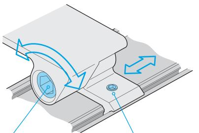
Tilt adjustment (3/16th / 4mm Allen wrench required)
