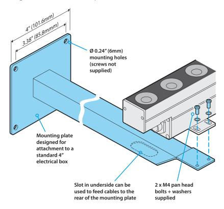
Note: When feeding cables through the extender bar check for any metal burrs that may have formed during manufacture - take care not to snag cables.
