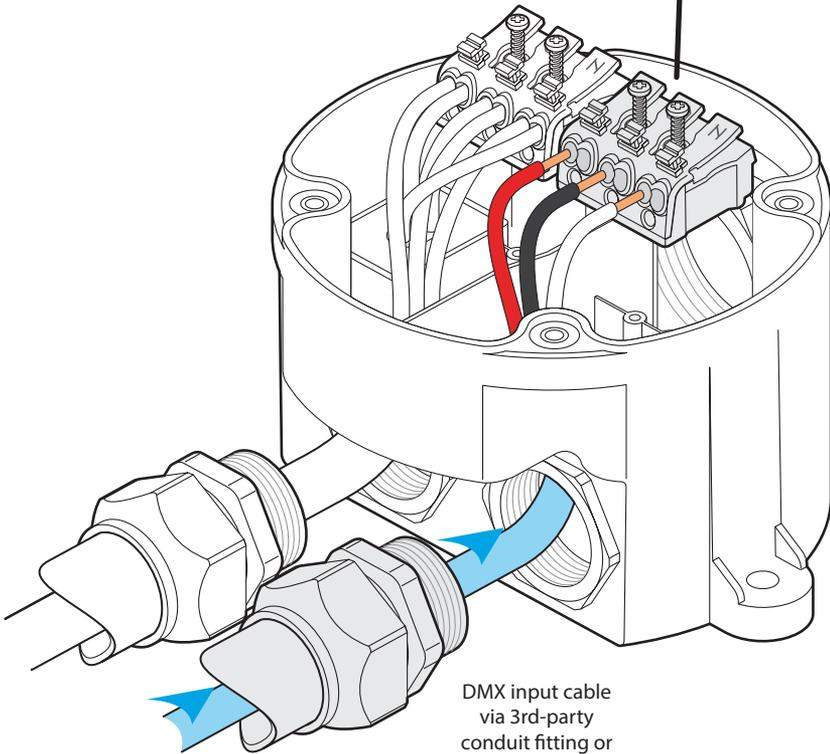
DMX input cable via 3rd-party conduit fitting or cable gland
