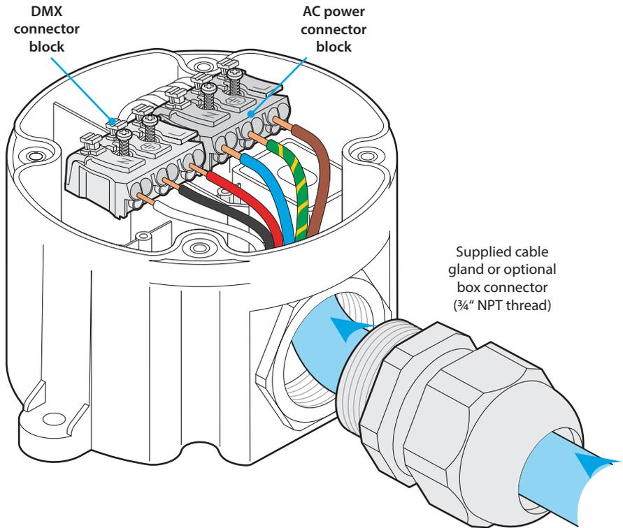
9 In turn, insert the six OLS feed wires into the AC power and DMX connector blocks, taking great care to ensure that the various wires are mated only with the correct terminals (see page 8 for wire designations):
