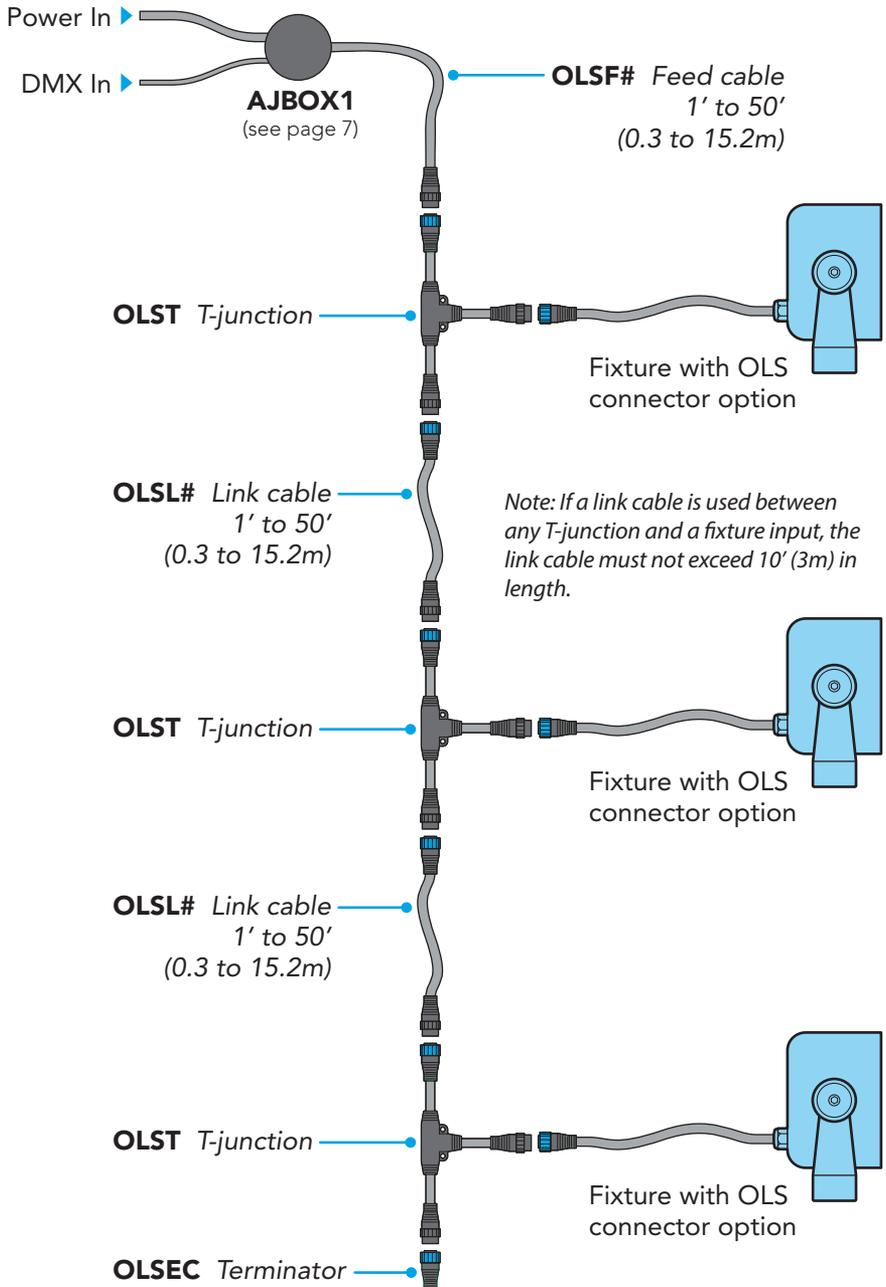
**IMPORTANT:** A terminator must be fitted to the final T-junction to simultaneously protect the live connections and correctly terminate the DMX control feed.
