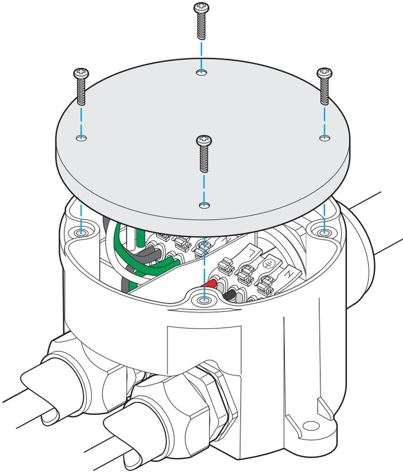
18 Use a #2 Phillips driver to secure the four screws to a reasonable hand-tightness.
