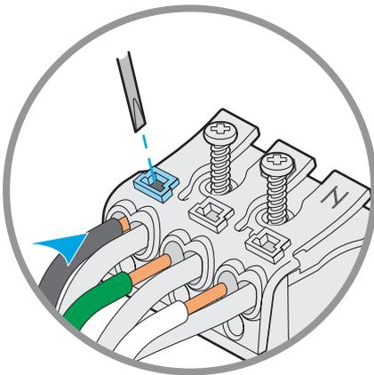
*Note: If the small buttons are not fitted to the connector block, insert a small flatblade screwdriver into each hole to open the spring contacts.*
