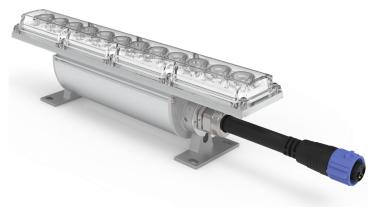
Linear XTR H1™ fixtures are precision engineered to deliver long runs of all-weather high-output linear illumination. When powered by standard mains (100 to 277VAC) they can achieve daisy-chained runs of up to 100 feet (30m). However, when supplied by an optional XTR Driver, the maximum length of a single daisy-chained run can be raised to 180 feet (55m).
