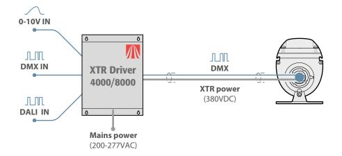
When using an XTR Driver, the internal conversion supports either a single 0-10V feed or a single 'broadcast' DALI channel - meaning that all Linear XTR H1 fixtures will use the same single control address. To benefit from multiple channels, use a ZDM 6 or DDC-1-AC to externally convert signals (see above).
