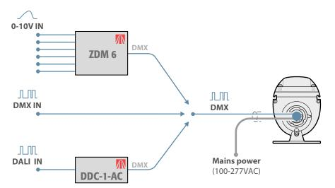
When using Acclaim Lighting ZDM 6 or DDC-1-AC modules it is possible to convert multiple inputs into separate DMX channels within a consolidated feed - thus allowing multiple Linear XTR H1 fixtures to be uniquely addressed. The ZDM 6 can convert up to six 0-10V inputs into DMX channels, whereas the DDC-1-AC can convert a maximum of 64 DALI channels (although large numbers of channels are not recommended due to the timing limitations of the DALI standard).
