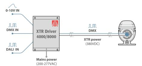
When using an XTR Driver, the internal conversion supports either a single 0-10V feed or a single 'broadcast' DALI channel - meaning that all Linear XTR fixtures will use the same single control address. To benefit from multiple channels, use a ZDM 6 or DDC-1-AC to externally convert signals (see above).
