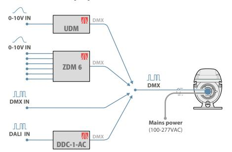
When using Acclaim Lighting ZDM 6 or DDC-1-AC modules it is possible to convert multiple inputs into separate DMX channels within a consolidated feed - thus allowing multiple Linear XTR fixtures to be uniquely addressed. The ZDM 6 can convert up to six 0-10V inputs into DMX channels, whereas the DDC-1-AC can convert a maximum of 64 DALI channels (although large numbers of channels are not recommended due to the timing limitations of the DALI standard).
