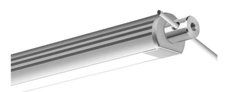
Flex Pendant Channel is a low profile double-anodized aluminum extrusion for mounting Acclaim interior Flex tapes. It can be suspended either from steel rods, stainless steel wire or alternatively surface mounted using brackets.
