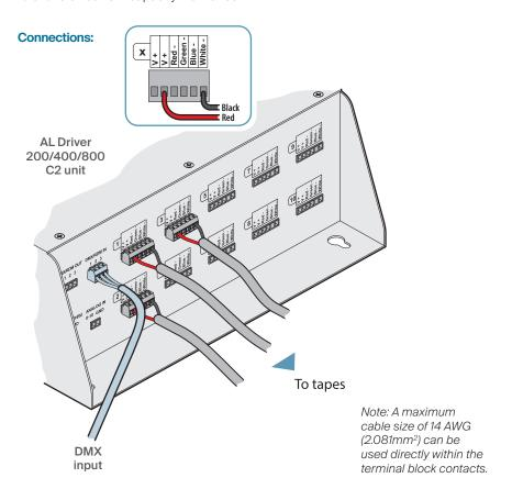
On all models, each port can support a maximum of **6.6A**, however, the maximum overall load across all ports must not exceed the following:
