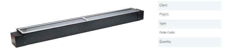
The **Dyna Exterior In-Grade System** allows you to place Dyna Graze or Dyna Cove Exterior runs directly in dirt or concrete. Troughs are constructed of epoxy coated stainless steel, with 3/8′ (10mm) tempered glass, and brushed stainless steel trims.
