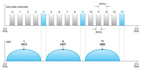
Where interference is suspected, a radio frequency survey may provide useful indications. If you have control over the nearest WiFi access points, it is suggested that you lock them down to one or more of the common channels (to prevent them from roaming) and select Aria channels that sit comfortably alongside.
