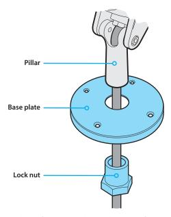
4 Secure the base plate to the surface/electrical outlet box using four suitable screws or bolts (preferably with countersunk heads).
