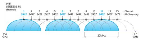
Aria uses the IEEE802.15.4 standard, with channels that are 3MHz in width and do not overlap. Many Aria channels do, however, coincide with the common WiFi channels. The notable exceptions are Aria channels 4, 9 and 14, which fall into the gaps between the most commonly used WiFi channels:
