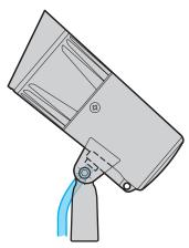
If the fixture will be tilted up, arrange the cable so that it exits at the front of the pillar.
