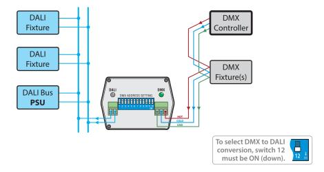
Note: For clarity, mains power inputs are not shown in the diagrams, but would be required at the controllers, the fixtures, the DALI PSU and the DDC-1-AC unit.
