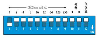
Note: Changes can be made to the switch settings while power is applied and the unit will respond accordingly.
