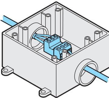
**Connections to the power cable are best protected within a junction box with suitable IP ratings**
