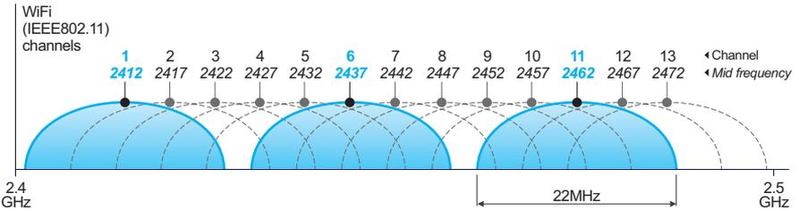
Aria uses the IEEE802.15.4 standard, with channels that are 3MHz in width and not overlapping. Many Aria channels do, however, coincide with the common WiFi channels. The notable exceptions are Aria channels 4, 9 and 14, which fall into the gaps between the most commonly used WiFi channels:
