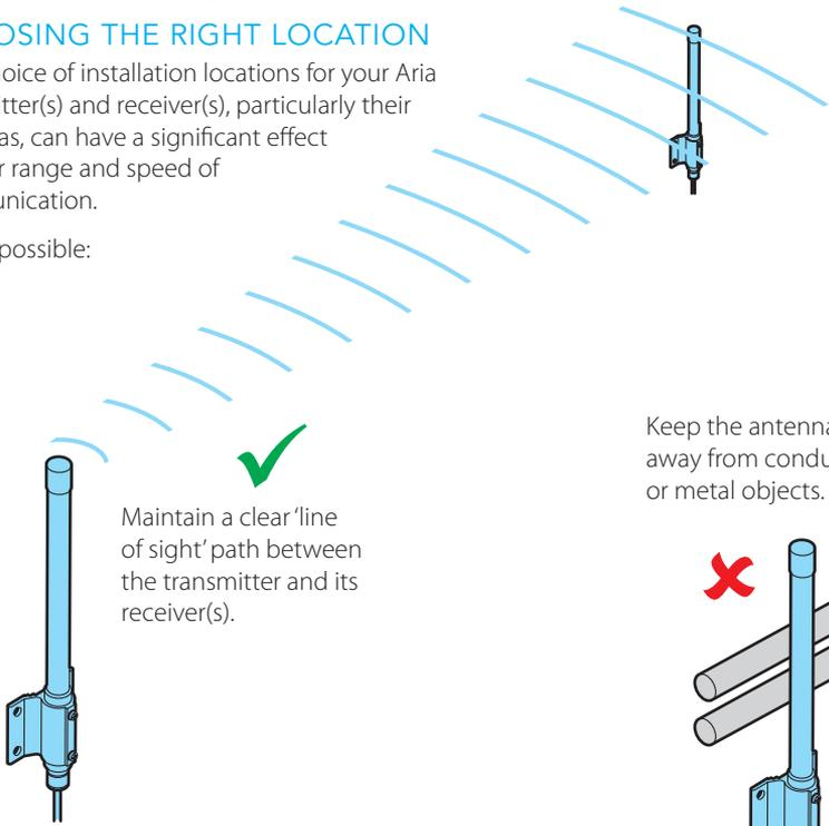
Maintain a clear 'line of sight' path between the transmitter and its receiver(s).
