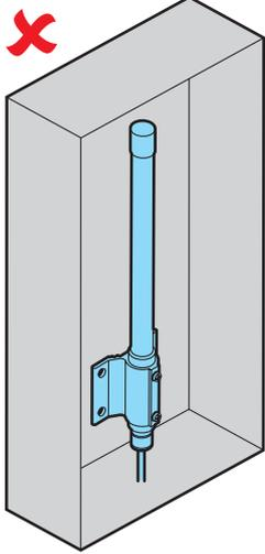
Keep the antenna at least 3 inches (75mm) from any surface such as walls, poles or the eaves of a building.
