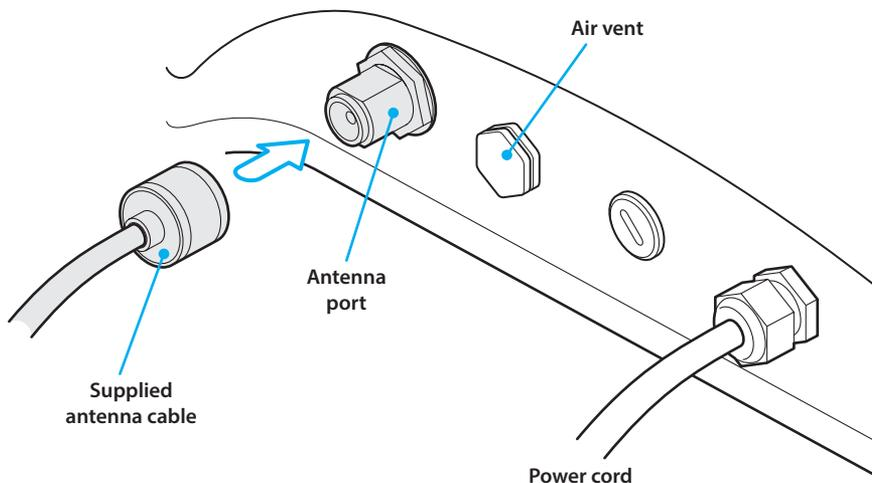
Alternatively, the antenna can be attached directly to the port on the Aria Range Extender underside, so that it hangs vertically downwards (the antenna bracket should be removed when using this method). This requires you to use the Type-N male to male adapter supplied within the package:
