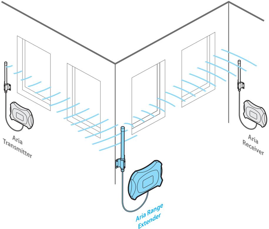
Ensure that the transmitter, receiver and range extender are all set to the same radio channel. The Aria Range Extender will receive the original signal, amplify it and re-transmit it.
