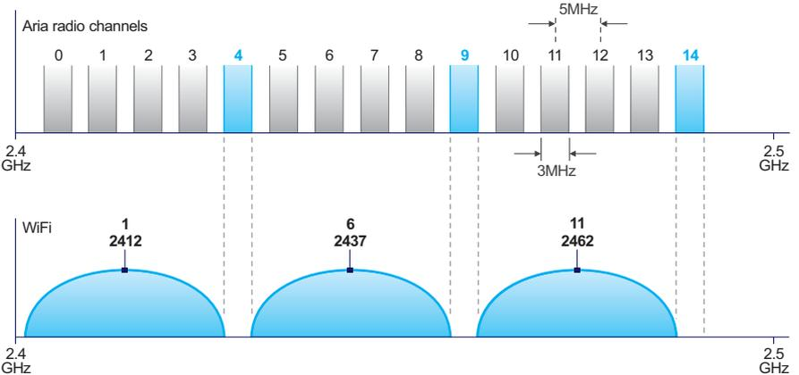
Where interference is suspected, a radio frequency survey may provide useful indications. If you have control over the nearest WiFi access points, it is suggested that you lock them down to one or more of the common channels (to prevent them from roaming) and select Aria channels that sit comfortably alongside.
