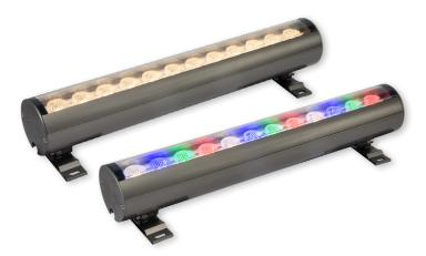
Aqua Graze™ fixtures are high output, submersible linear LED fixtures suitable for use in all aquatic locations down to a depth of 10' (3m). A range of emitter types, lens options and full UL676 Pool & Spa certification make these fixtures particularly suited for exterior façade washing as well as fountain, pond and landscape applications.
