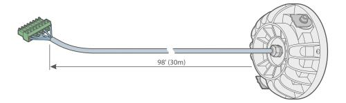
In situations where the Aqua Drum cable is connected to a supply cable before arriving at the driver, ensure the conductors of the supply cable are of sufficient size and that the total cable length (including the Aqua Drum cable) is not exceeded:
