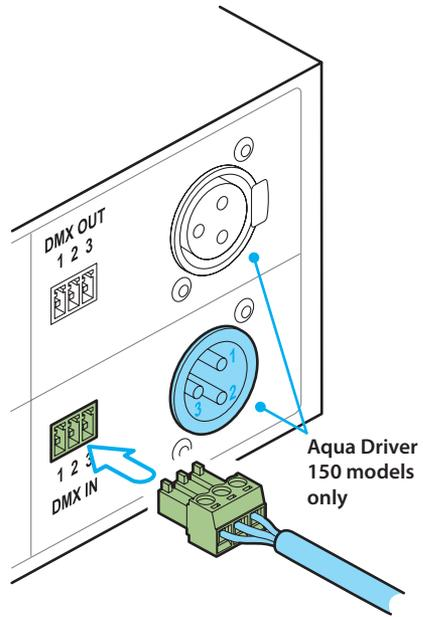
Insert the terminal block into the DMX socket and ensure that it fully clicks into place. Repeat for the DMX OUT if the control signal needs to be fed to another device.
