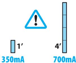
**IMPORTANT:** 1’ fixtures require a different drive current setting to the longer 4’ fixtures - it is vitally important to select the correct setting to avoid damage to the fixtures. The drive current setting affects all outputs equally, so it is not possible to mix the two sizes on the same driver unit. See “Fixture drive current selection” on page 9.
