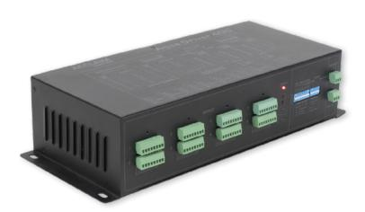
Aqua Driver 400™ is a constant current dimming driver for 24VDC-based fixtures, including the Aqua Drum and Aqua Graze ranges. Smooth dimming is provided for up to eight RGBW/A, Dynamic White or Fixed White fixtures under DMX control. Additionally, static colors and adjustable chases can be configured when independent operation is required.
