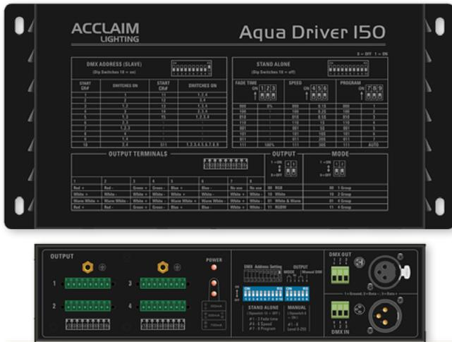
**Aqua Driver 150™** is a constant current dimming driver for 24VDC-based fixtures, including the Aqua Drum and Aqua Graze ranges. Smooth dimming is provided for up to four RGBW/A or single-color fixtures under DMX control. Additionally, static colors and adjustable chases can be configured when independent operation is required.
