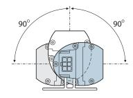
Each swivel mount base has two slots measuring Ø0.18 x 0.39" (Ø4.5 x 10mm) on 1.65" (42mm) centers. The mount bases have a thickness of 0.08" (2mm). Select bolts or screws (not supplied) which fit the swivel mount base(s) correctly and are particularly suited to the mounting surface.
