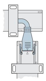
Take care not to stress the cable when connecting in this way. Use optional link cables to achieve greater separation/angles.
