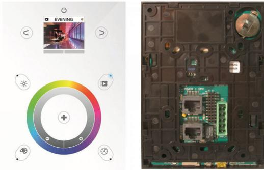
The **Art 500** is a touch panel DMX Controller with 1,024 DMX channels and 500 programmable scenes, designed to be the most effective control solution for architectural control. Included is the ART 500 software package, which offers an easy to navigate interface, combined with powerful control features.
