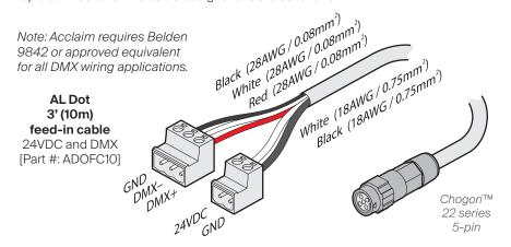
IMPORTANT: These connectors are not rated for live connection or disconnection. Check that power is isolated before making or breaking any links. Ensure the connectors have locked and are seated correctly before applying power.
