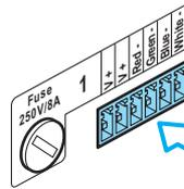
Insert the terminal block into the required output socket and ensure that it fully clicks into place.
