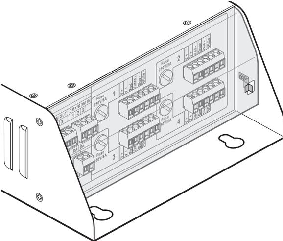
2 Disengage the upper lip of the cover from the AL Driver frame.
