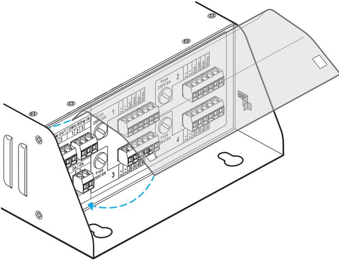
2 Lower the lower edge of the cover down so that the two holes align with the two clips located on the driver side walls.
