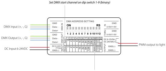
Dip switch 10 on (up) to activate DMX input
