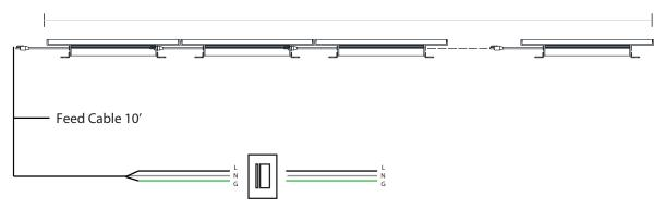
Compatible with most forward phase (TRIAC) dimmers For 0-10V or DMX control use an external UDM
